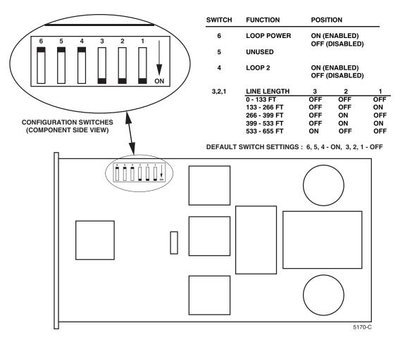
Figure 516-1. Version C HLXC Module Configuration Switches
